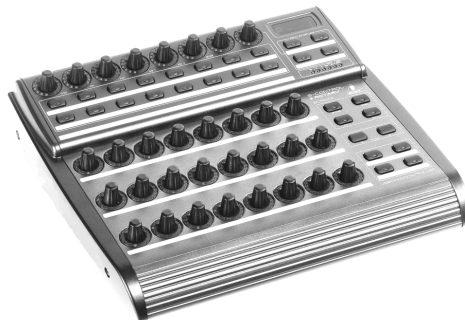
Fig. 5. Examples of a potentiometer board. Midi controller boards, such as the one shown here, can be modified so that their rulers (here potentiometers) directly change the neuron activity of associated local neurons. These neurons are accessible from all control boards of the Myon robot via communication bus and can be used to influence the network dynamics.
