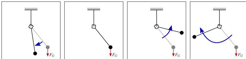
Figure 2. Different behavioral modes of the CSL form nature-like motions; From left to right: release, hold current position, contract, or support an externally induced motion.
