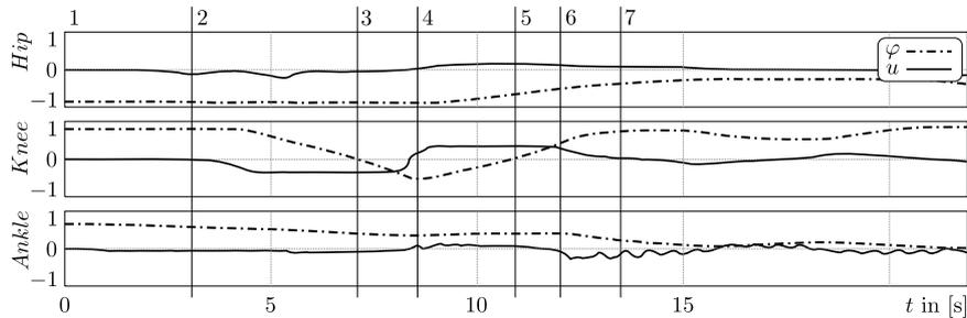
Figure 4. Joint angles of Myon's leg and the control outputs in the stand-up motion. The numbered vertical lines correspond to the snapshots of Figure 3. An experimental run takes about 20 seconds. In the end (7) the leg is never at rest but performs a slight swinging motion in upright position.
