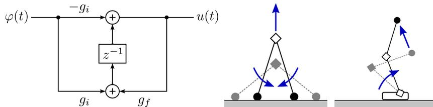
Figure 1. Left: Structure of the CSL. Right: CSL operating in contraction mode for different morphologies which are subjected to gravity.
