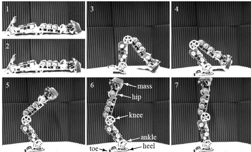
Figure 3. A single leg of the modular humanoid robot Myon standing up using the proposed CSLs. Each of the three joints is locally controlled by a contracting CSL whilst no direct communication takes place between the controllers. Complex behavior emerges from the interplay via momentum.
