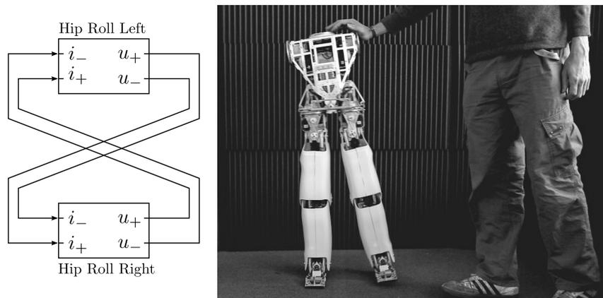
Figure 5. Left: Schematic view of crossed inhibitory connections between two CSLs controlling left and right hip motors of a humanoid robot. Right: Lower body part of Myon during balancing motion. Head and Arms are not attached. Contracting CSLs on the hip joints make the body withstand pushes or adapt its upright posture to tilted grounds.
