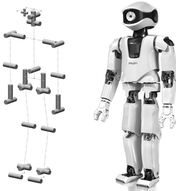
Figure 1. The humanoid robot MYON. Left: Schematic diagram of the joints' positions and orientations. Right: Image of the functional robot including the exoskeleton shells. The exoskeleton is a structural element which prevents the inner endoskeleton from external torsional loads. Furthermore, the electronic components are protected from mechanical impacts and the user from crushing injuries.
