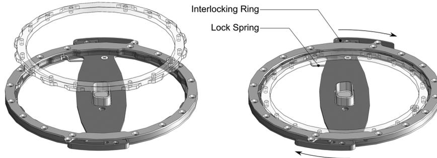
Figure 4. Detailed view of the novel flange which firmly connects the robot’s body parts mechanically, whilst at the same time relaying the power supply lines and sensorimotor signals. The flange can be controlled using a single hand and allows for detachment and reattachment of body parts during runtime.
