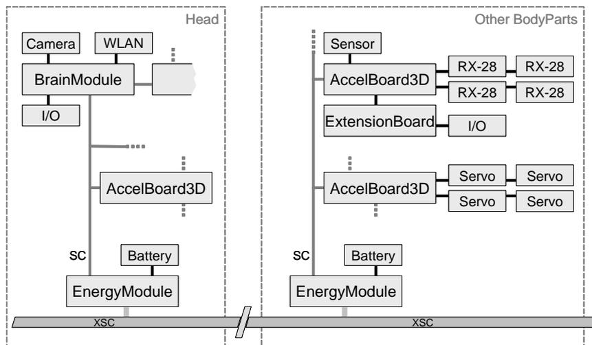
Figure 2. System architecture of the robot MYON. Components within each body part are connected via the so-called *Spinal Cord* (SC), whereas the body parts are connected by the *Extended Spinal Cord* (XSC) which includes several additional lines for energy transfer as well as a control line for quick shutdown of the robot.
