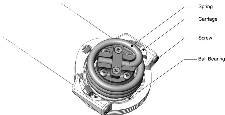
Figure 6. Detailed view of the torsion spring which is connected to each actuator in a compact way. The spring provides the necessary series elasticity to drive a single joint with multiple actuators in an antagonistic way. Forces are transmitted via wire ropes (also see Figure 7) which are clamped by a screw. Additionally, the spring also protects the actuator's gear from unforeseen high external impact forces.
