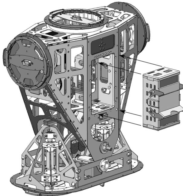
Figure 3. Construction of the robot's torso, exhibiting the flanges for the other body parts. The torso is made of aluminum and therefore only weighs 2.5 kg including actuators, electronics and batteries. The design of the battery pack allows for easy insertion and removal using a single hand.
