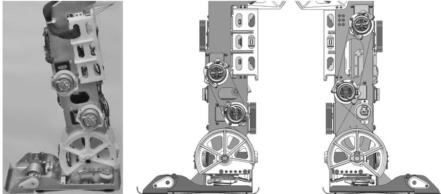
Figure 7. Detail of the ankle joint. Left: Photograph of the foot and leg without exoskeleton shells. Middle and Right: Schematic side views showing the four actuators (small circles) which drive the ankle pitch joint (big circle) via wire ropes.
